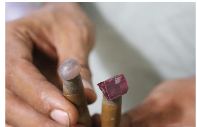
ABOVE: Rubies fixed on a dop stick at two stages of cutting. LEFT: Artisan Daud ustaz shows individual facets on a tourmaline.
